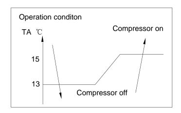
6.6.1.1 When TA<13°C, the compressor stops working. And the outdoor fan will stop delaying for 5
