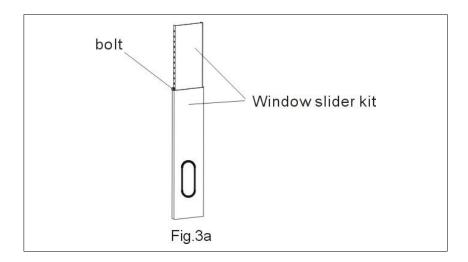
Note: If the window opening is less than the mentioned minimum length of the window slider kit, cut that one with a hole in it short to fit for the window opening. Do never cut out the hole in window slider kit.
